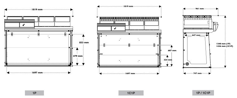
Please add 150mm between the last filter and the ceiling to allow good air recirculation and to replace filters easily
