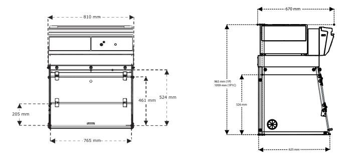
Please add 150 mm between the last filter and the ceiling to allow good air recirculation and to replace filters easily.
